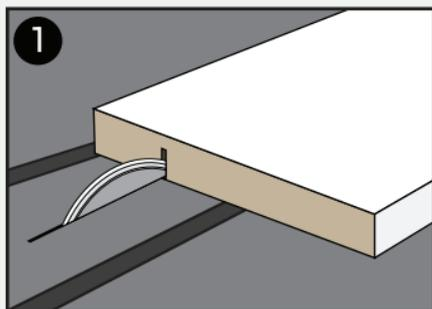
Cut a  $\frac{7}{32}$ " (6mm) slot in the rear of trim to the desired gap height.
