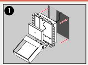
Remove Door and Mounting Plate. Dry fit **Body** into place. Ensure wiring is run through the hole.
