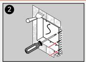
Fasten **Body** in place with screws. Mud and tape drywall compound to cover flange.
