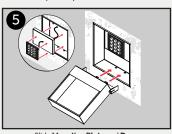
Slide **Mounting Plate** and **Door** back into place.
