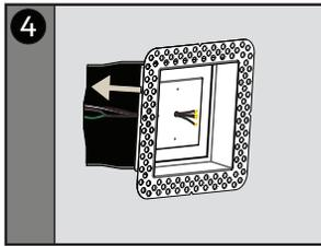
4 Feed wires through pre-drilled hole and place the **Mount** in the cavity.
