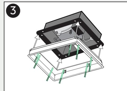
Mount fan to top of **Framed Exhaust Mount** and secure with **screws**.
