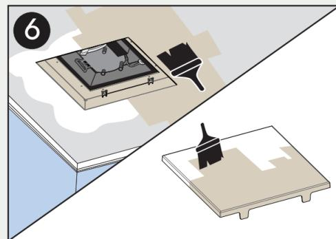
Paint inside of body, faceplate, and surrounding drywall. Wallpaper can also be used. Do not paint fan.
