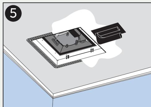
Use drywall compound mud to cover flange surface. Once dry, sand. Repeat as necessary.
