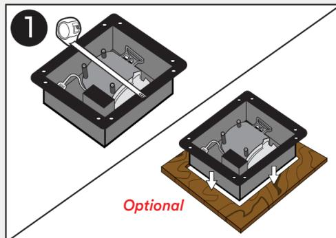
Measure ventilation fan to ensure fit. If fan is smaller than the opening in **Framed Exhaust Mount**, use plywood as an adapter to increase flange size.
