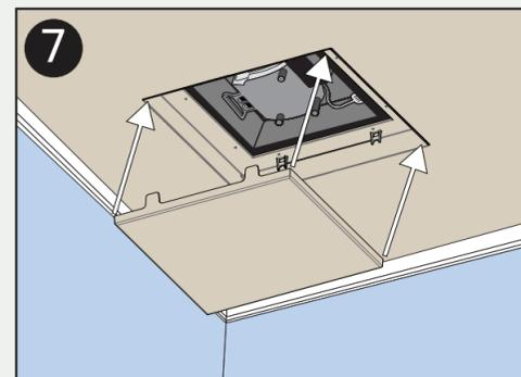
Align tabs on body and faceplate, push to snap into place.
