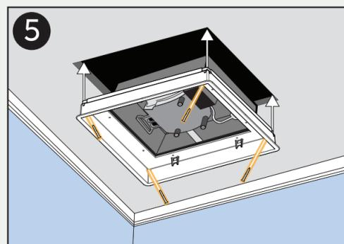
Dry fit **Framed Exhaust Mount** into cavity. Secure four inner corners to ceiling frame using included **wood screws**.
