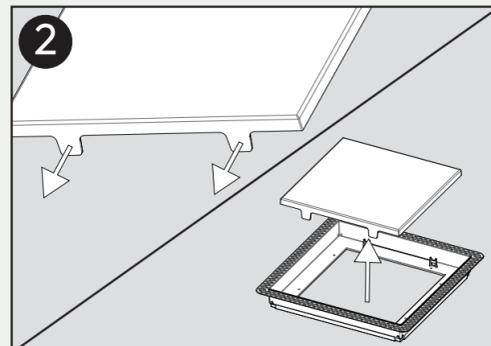
Disengage faceplate of **Framed Exhaust Mount** by pulling legs outwards.
