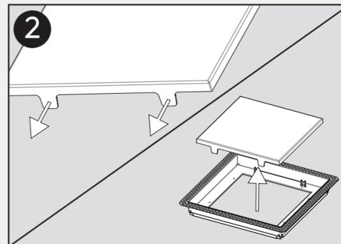
Disengage faceplate of **Flush Exhaust Mount** by pulling legs outwards.
