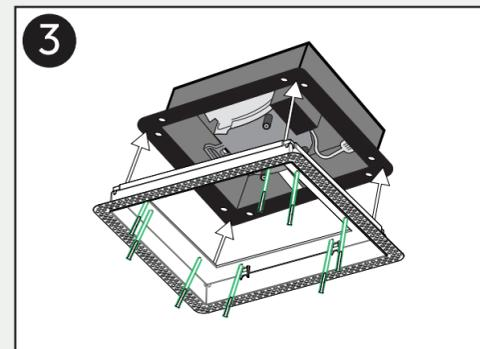
Mount fan to top of **Flush Exhaust Mount** and secure with **screws**.
