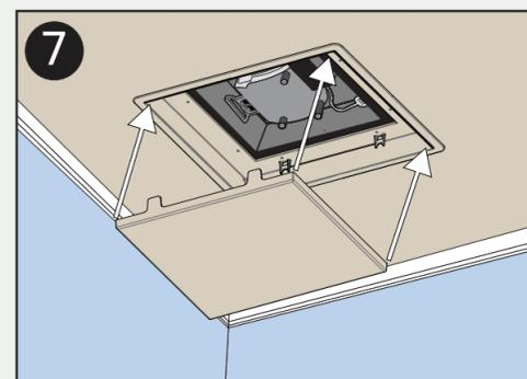
Align tabs on body and faceplate, push to snap into place.
