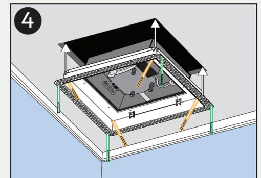
Dry fit **Flush Exhaust Mount** into cavity. Secure four inner corners to ceiling frame using included **wood screws**. Add **drywall screws** on bead as necessary.
