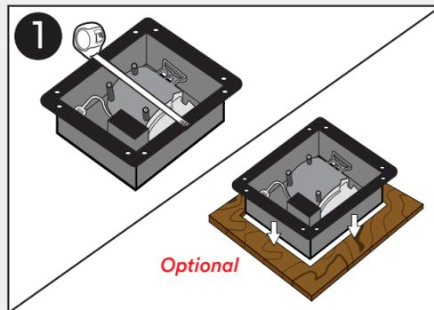
Optional: Measure ventilation fan to ensure fit. If fan is smaller than the opening in **Flush Exhaust Mount**, use plywood as an adapter to increase flange size.
