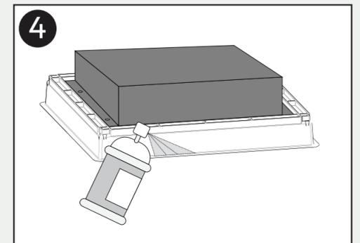
Use adhesive on back of Frame to stick **Framed Exhaust Mount Body** to the opening.
