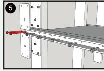
Fasten with provided screws. 2 additional long screws required (not included).
