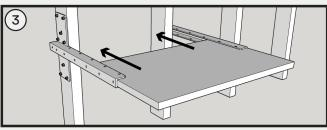
Slide in structural board. Must fit snug with minimal movement.
