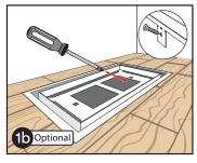
Secure vent with screws.
