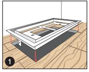
Dry fit Aria Vent body piece in opening.
