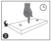
Flip tray and allow bonding material to cure. Ensure flooring material is flush with the rim.
