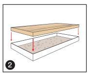
Apply adhesive bonding material in tray. Insert pre-cut flooring material.
