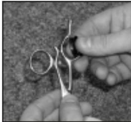
1. When bending the handle on a pair of shears, always start by removing any ring sizers from the finger or thumb holes.
