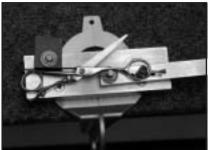
5. Make sure the open blades have good contact with the neoprene block before you start bending.
