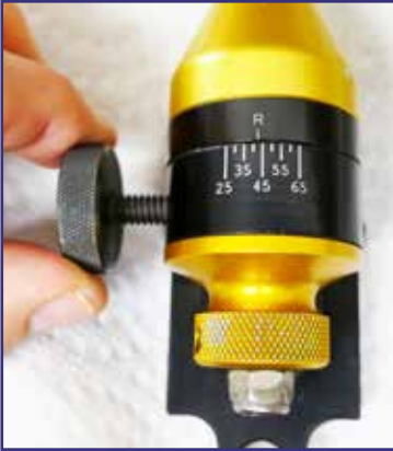
Loosen the Angle Lock Knob
