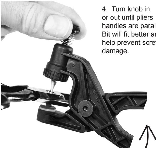
4. Turn knob in or out until pliers handles are parallel. Bit will fit better and help prevent screw damage.
