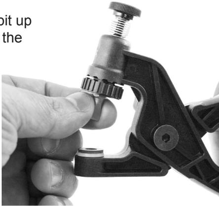
3. Place scissors on anvil and rotate ratchet to align bit with screw. Close pliers firmly to force blade and ratchet into position.
