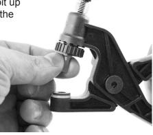
3. Place scissors on anvil and rotate ratchet to align bit with screw. Close pliers firmly to force blade and ratchet into position.
