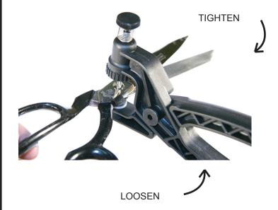
6. The best way to set the free fall is to hold the shears firmly in the pliers and open and close the shears using the shears handle directly beneath (under) the screw head. This handle usually pivots freely.
