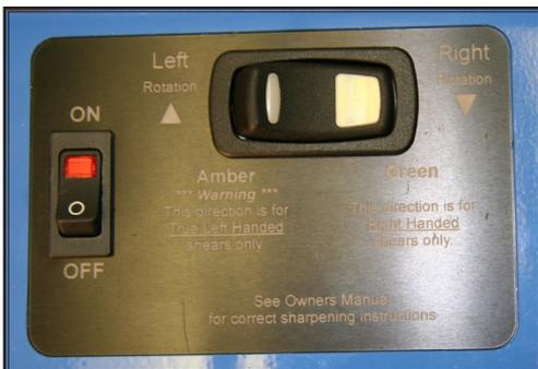
Plug machine into a 3 wire grounded receptacle only. Make sure the direction switch is in the right hand scissors position. Turn on the the power switch and stand aside and let it run for one minute before using it the first time. Follow this step also after replacing the corrugating wheel.
