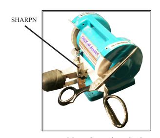
Move sharpening wheel to right hand side of sharpener and honing wheel to left hand side.
