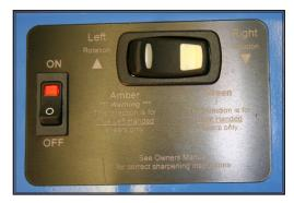
Plug machine into a 3 wire grounded receptacle only. Make sure the direction switch is in the right hand scissors positon. Turn on the the power switch and stand aside and let it run for one minute before using it the first time. Follow this step also after replacing the corrugating wheel.
