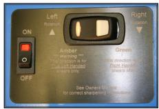
WARNING - The blade will move from the tip to the pivot this is the opposite direction of movement when you are doing a right hand scissors
