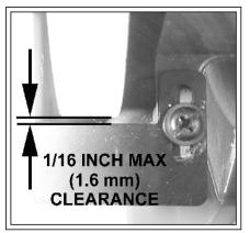
As the wheels wear adjust the two finger and two tongue quards to maintain the maxium 1/16 inch between the wheels and the guards.
