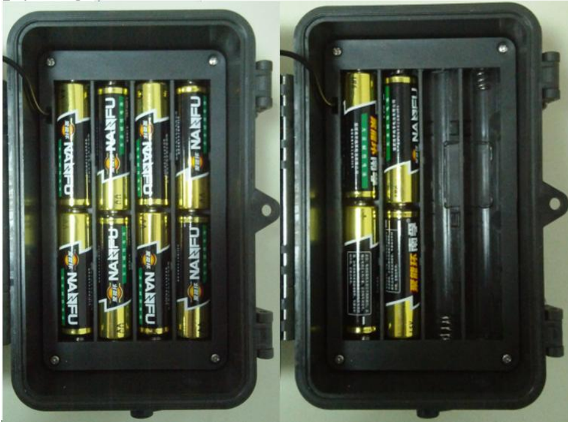
Fig. 5: Battery Configurations of 8 or 4 batteries
