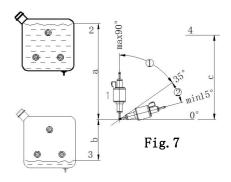
a  $\leq$  3m b  $\leq$  0.5m (Avoid of negative pressure may be produced in sealed fuel tank. In such case, b  $\leq$  0.15m) c  $\leq$  2m.
