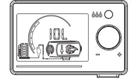
When you fulfill your tank you can reset the fuel gauge by pressing the "Fuel volume settings key".
