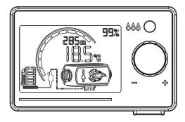
adjustment can be achieved by short pressing the "+" or "-" button on the Wireless Remote Controller. After a few seconds the buzzer will beep once as settings confirmation.
