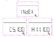
C5.1000-- LCD switch version H11.100-- master controller version
