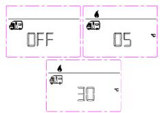
Flame icon = room temperature heating start, this icon will flash until the predetermined room temperature is reached.
