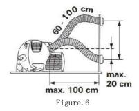
After the intake and exhaust pipes are pierced from the through holes, they must be cut short, and the exhaust pipes are slightly shorter than the intake pipes. Avoid excessive expansion or tension on the exhaust pipe.
