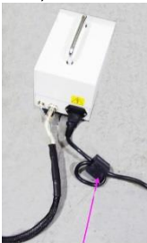
Ferrite bead (with 2 turns) on AC mains cable
