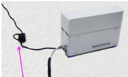
Ferrite bead (with 2 turns) on interconnection cable
