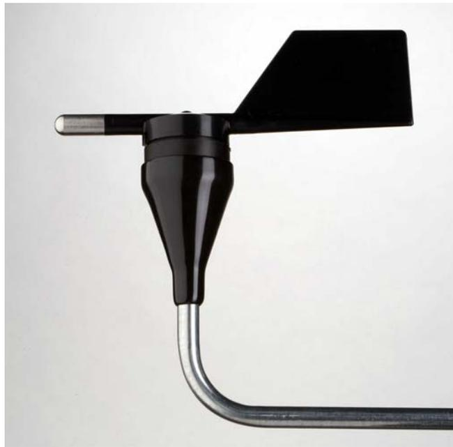
The #200P wind direction vane is the industry standard wind direction vane used worldwide. The thermoplastic and stainless steel components resist corrosion and contribute to a high strength-to-weight ratio. The vane is directly connected to a precision conductive plastic potentiometer located in the main body. An analog voltage output directly proportional to the wind direction is produced when a constant DC excitation voltage is applied to the potentiometer. A rubber terminal boot is included.
