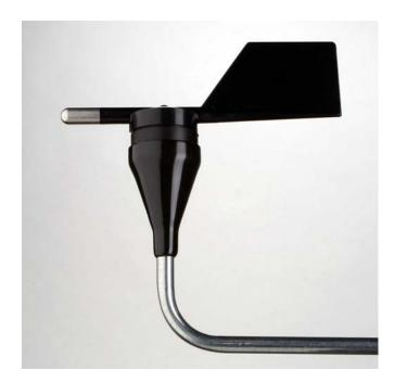
The #200P wind direction vane is the industry standard wind direction vane used worldwide. The thermoplastic and stainless steel components resist corrosion and contribute to a high strength-to-weight ratio. The vane is directly connected to a precision conductive plastic potentiometer located in the main body. An analog voltage output directly proportional to the wind direction is produced when a constant DC excitation voltage is applied to the potentiometer. A rubber terminal boot is included.
