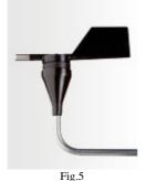
The data logger also has to have suitable software to averaging the results, so that the "north jump" can be accounted for: the average of 350° and 10° should result in "North" and not 180°!
