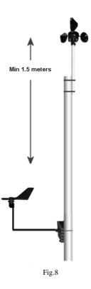
Spiral wraps sensor cables around the tower, one wrap per tube joint. The spiral promotes vortex shedding and reduces natural frequency oscillations of the tower. Use electrical tape to tape the sensor cables and ground cab to the tower every few meters. Also tape cables to the tower above and below each guy ring. Where the cables cross each guy ring, protect the cables by wrapping them with a thick layer of electrical tape as shown below.
