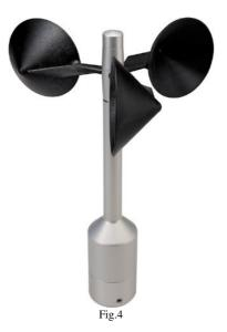
Opto-electronic transformers and AC-generators have proved to be the most suitable transducers for its robustness.
