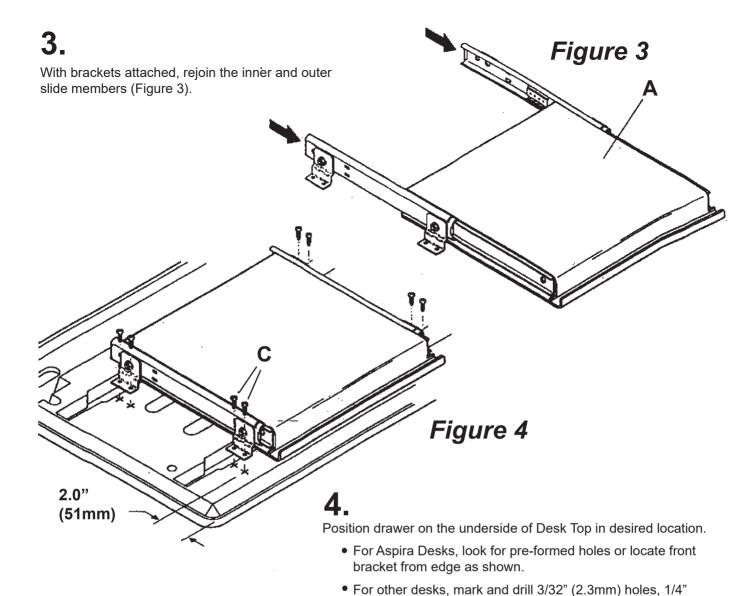
Attach drawer with Screws (C) as shown in Figure 4.
