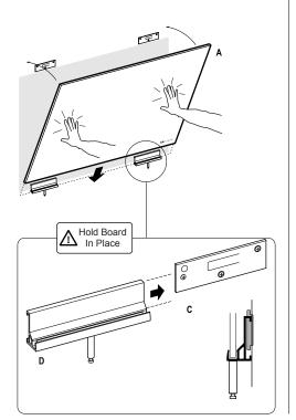
While holding board in place, carefully slide top support brackets (2X) over the secured mounting plates.
