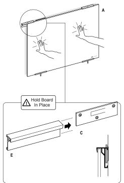
4 Slide the single **rail** through the bottom post of support bracket at a slight angle. Then rotate rail and slide through opposite post. Adjust rail so that it is even.
