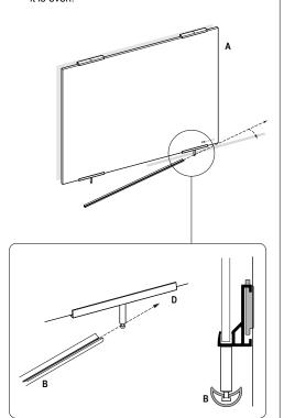
5 Turn plastic sleeve on **post** to secure rail to bottom brackets. Take the **eraser tray** and secure it to rail at desired location.
