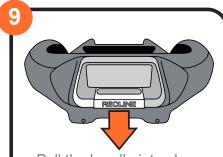
Pull the handle into place until you hear a snap. Then pull the handle forward and release to snap it back into place.
