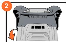
To re-assemble; stand the base on end so the front of the base is facing upward. Press down on one side to release the recline foot.
