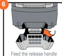
Feed the release handle upward toward the release handle opening and hold in place.
