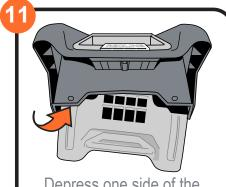
Depress one side of the recline foot and press it into the base to join the corresponding fittings.
