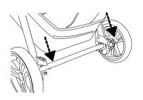
8) • To engage rear brakes, apply downward pressure to the brake levers located on the rear axle. The stroller may require forward or rearward movement in order to engage the brake. Check that the stroller will not move once the brakes are properly applied. To release, gently lift up on the brake levers (Fig. 8).
