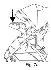
7) · To attach the child tray: Push the tray downward and onto each side of the front armrests until both sides snap into place (Fig. 7a). Check that the tray is secured by
