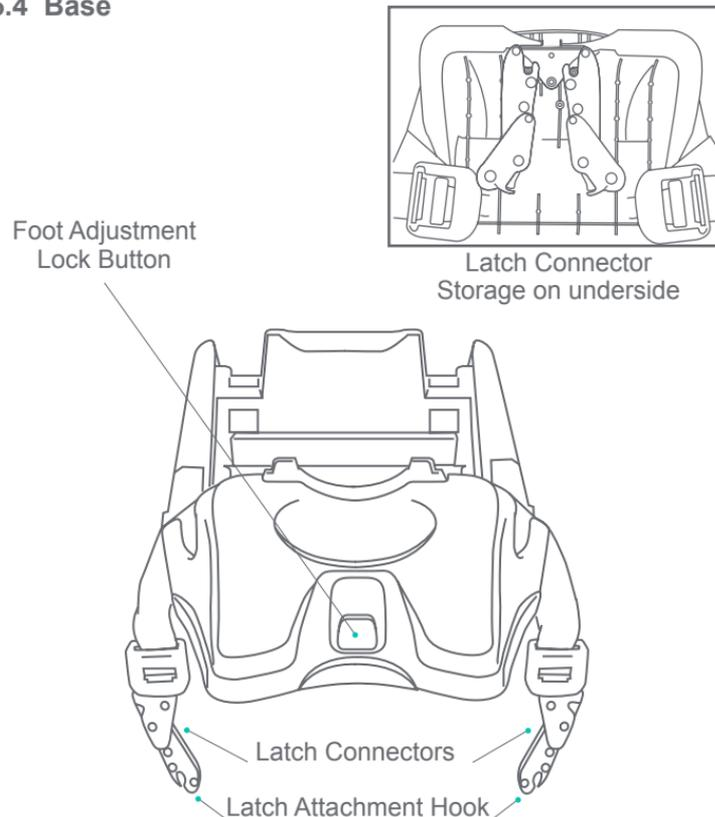
Your Safety Seat base can be installed with either the vehicle belt or with the included LATCH attachment system.
