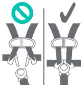
Children have **STRANGL**ED in loose or partially buckled harness straps. Fully restrain the child even when carrier is used outside the vehicle.
