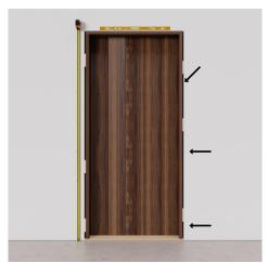
**Step 9.** Check both sides of the jamb for plumb again with a level.
