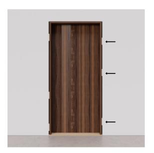
**Step 4.** Set shims around door unit for a tight fit.
