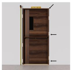
**Step 9.** Check both sides of the jamb for plumb again with a level.
