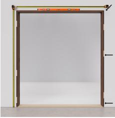
Step 5. Place the jamb and threshold in the opening, securing with shims for a snug, even fit. Confirm it's square by ensuring diagonal corner-to-corner measurements
