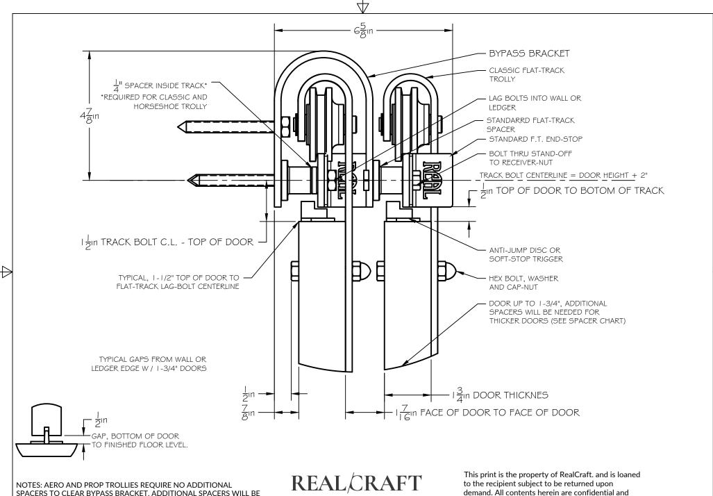
NOTES: AERO AND PROP TROLLIES REQUIRE NO ADDITIONAL SPACERS TO CLEAR BYPASS BRACKET. ADDITIONAL SPACERS WILL BE REQIRED ON OUT-SIDE TRACK FOR 2-14" AND THICKER DOORS TO ALLOW FOR DOOR CLEARANCES (BETWEEN DOORS).
