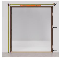
Step 5. Place the jamb and threshold in the opening, securing with shims for a snug, even fit. Confirm it's square by ensuring diagonal corner-to-corner measurements match. Check jamb legs for plumb with a level so your doors are easier to hang.
