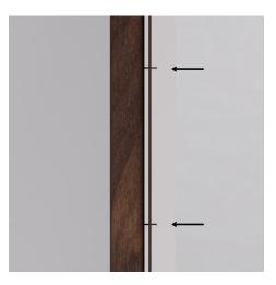
Step 11. Attach the astragal over the gap between the doors using screws, centering it for an optimal fit.
