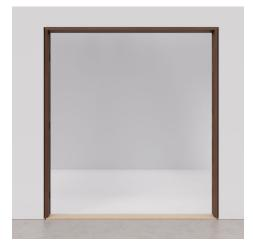
**Step 4.** Test fit the jamb in the rough opening. Lay several thick beads of adhesive silicone below the threshold before installing.
