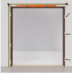
Step 5. Place the jamb in the opening, securing with shims for a snug, even fit. Confirm it's square by ensuring diagonal corner-to-corner measurements match. Check jamb legs for plumb with a level so
