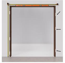
**Step 4.** Use mallet to ensure the unit is plumb. Check with a level and measuring tape to ensure that the unit is square and plumb. Secure jamb with at least one screw 3 inches long behind the weatherstripping at the top hinge and bottom hinge.
