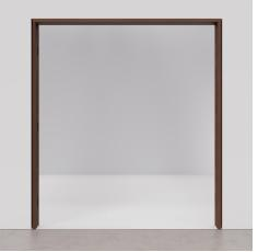
Step 3. Place the jamb in the opening, securing with shims for a snug, even fit. Confirm it's square by ensuring diagonal corner-to-corner measurements match. Check jamb legs for plumb with a level so your doors are easier to hang.
