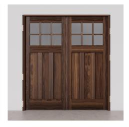
Step 7. Ensure the doors fit correctly by closing them and adjusting shims for the best fit and even gaps. Maintain an equal gap between door slabs at top and bottom. Adjust using shims/hinges until gapping is uniform. Finally, check for any binding issues.
