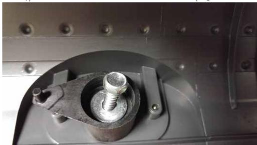
2. Remove the screw, washer, pin shaft, and spacer washer revealing the black cam ring
