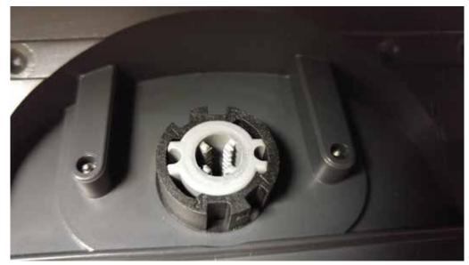
4. The Cam Ring is free spinning so to adjust, simply move it left or right. Simply by adjusting which set of notches are at the 12:00 and 6:00 positions, determines which direction the play is on the pin lever
