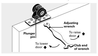
Note: The top of the hanger shaft screws into a self-locking nut. If the hexagonal nut is turned downwards too far, the shaft will become loose from the self-locking nut. If the turning resistance suddenly feels much easier, you have gone too far.
