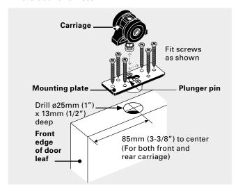
d) Mount bearings at the bottom of each door using the screws supplied.
