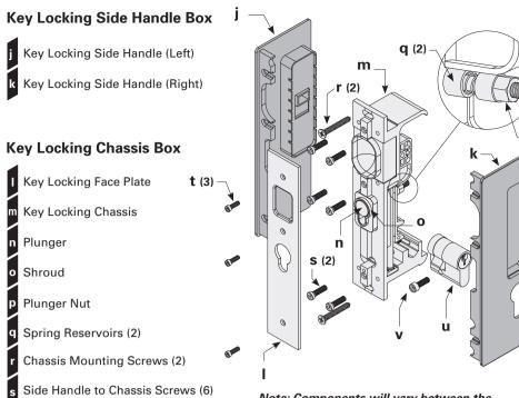
Note: Components will vary between the 'Key One Side', 'Key/Key' and 'Key/Snib' versions.
