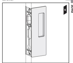
**7**. Fit the *Bi-Parting face plate* to the chassis using the 3x *handle face plate screws*.
