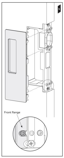
**6.** Fit the remaining Bi-Parting side handle to the chassis and tighten the side handle screws.
