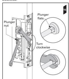
**16**. Continue to turn the spanner until there is no longer a gap between the spanner and the shroud face.
