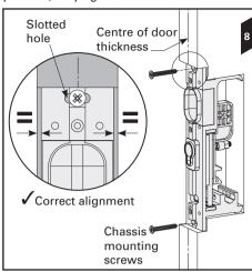
9. Fit the 6x side handle to chassis screws. Leave a 3mm gap (1/8") between the underside of the screw head and the chassis.
