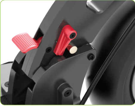
QUICK FOLDING MECHANISM SELF LOCKING / RELEASE BUTTON
