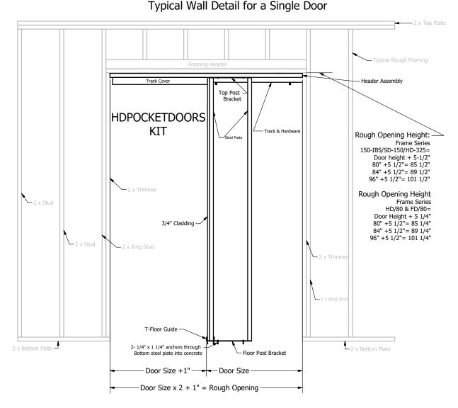
HDPOCKETDOORS fabricates standard sizes of heavy duty pocket door frames for 2x4 and 2x6 walls for 80", 84", and 96" door height and 48"- (and smaller) door width. With ample lead time, custom frame kits can manufactured for any height, width, and wall thickness for any application.
