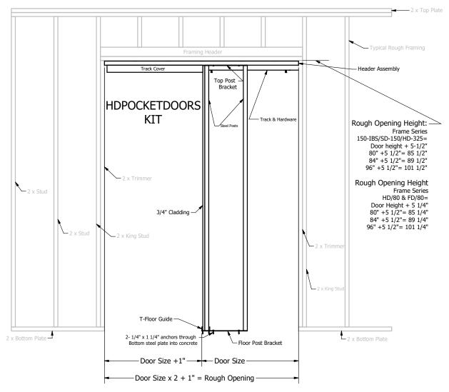
HDPOCKETDOORS fabricates standard sizes of heavy duty pocket door frames for 2x4 and 2x6 walls for 80", 84", and 96" door height and 48"- (and smaller) door width. With ample lead time, custom frame kits can manufactured for any height, width, and wall thickness for any application.
