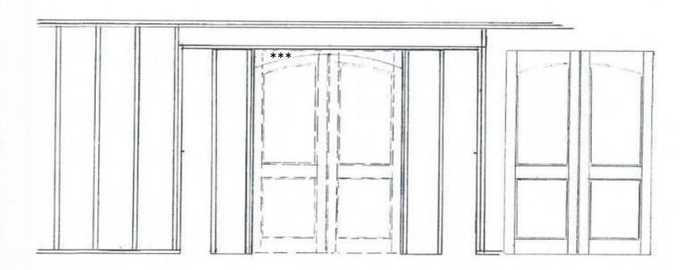
A custom order will have the LVL Head in one piece with the converging block in place. Two single door kits could be used by adding a converging block.
