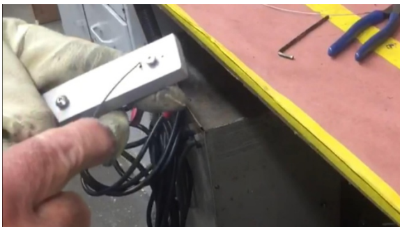
5. Insert the other end of the wire into the small hole in the other end of the tool and pull it through. The smaller hole is for gauges 12 through 17, and the larger for heavier gauges.
