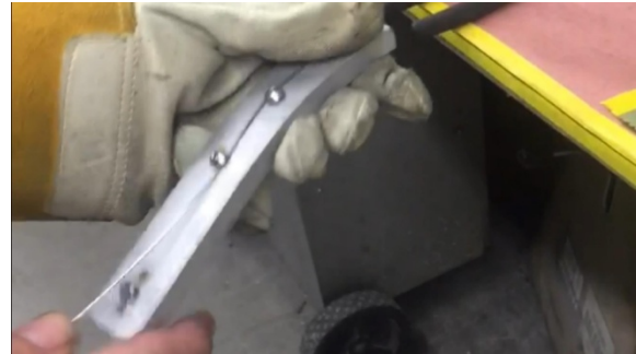
2. Secure wire under the screw heads.
