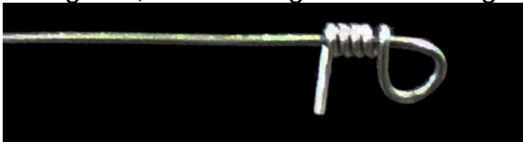
7. Trim the excess tail of the loop.
