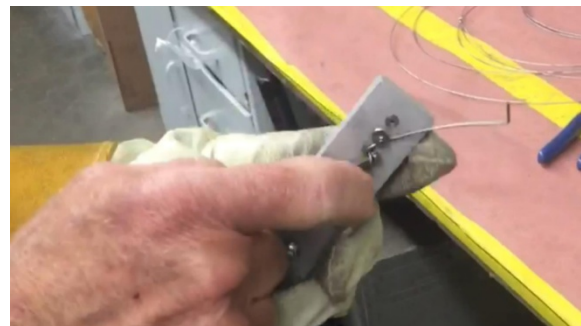
6. Using a screwdriver or other tool with a shaft that is roughly 3/16" through the loop, rotate counterclockwise to wind the loop, with the tail of the loop under the screw as shown.
