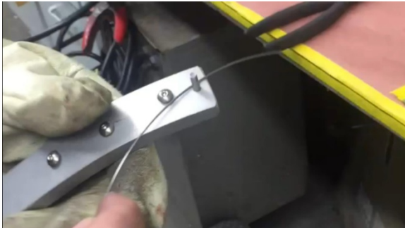
1. Place wire to the left of the pin.
