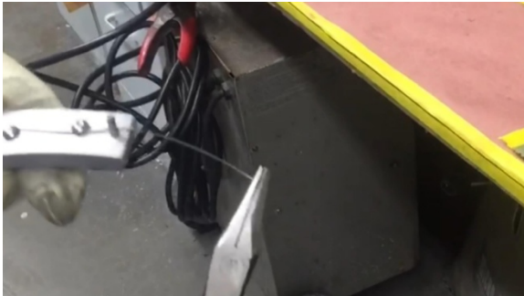
3. Make 90 degree upward bend at end of wire.
