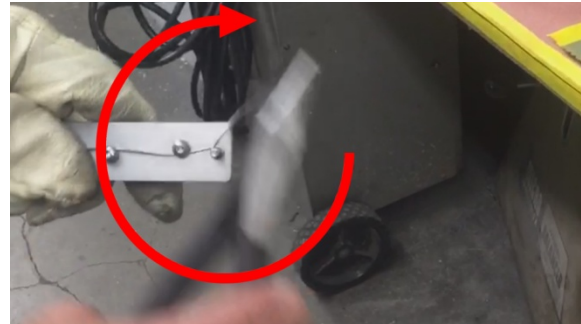
4. Loop around the pin 270 degrees, or 3/4 turn, going a bit further so the wire ends up perpendicular to the tool when it springs back.
