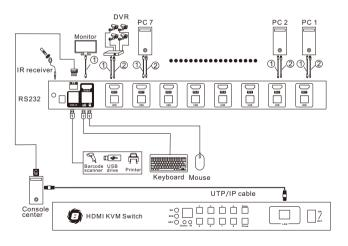
Note: ① HDMI cable ② USB type A to USB type B cable
