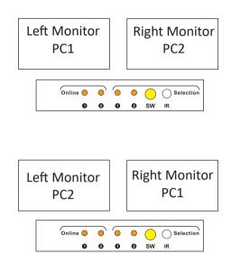
PC1 displays on 1 monitor and PC2 displays on other monitor, simultaneously.
