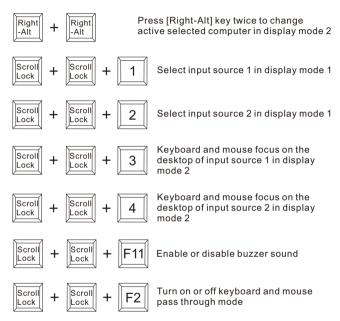
**Note**: For the best compatiblity, it is better to turn on keyboard and mouse pass through mode. In this mode, the keyboard and mouse are dynamically mapped to computer, so you are able to use special keyboard and mouse that with multimedia keys or other customized keys.
