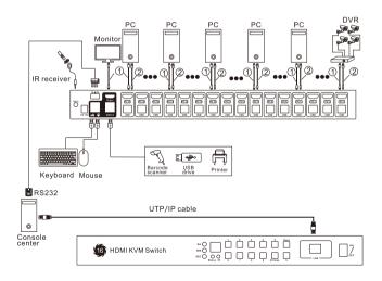
Note: ① HDMI cable ② USB type A to USB type B cable
