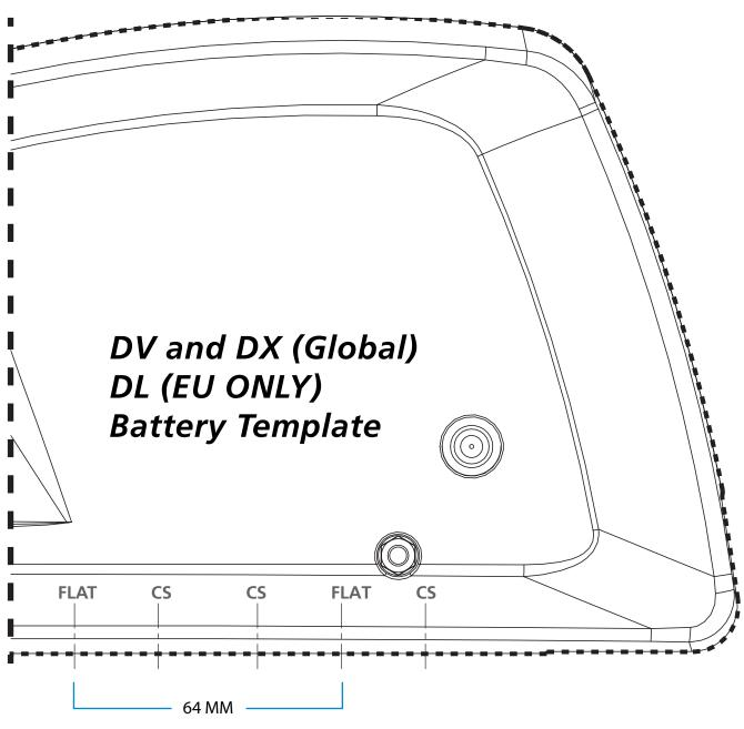
Flat = Flat holes and button head screws CS = Countersunk screws and holes NO = Do not use for alignment (OEM only)
