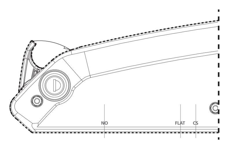
Cut out the battery template, use the markings over the bottle cage holes on the bicycle frame. The flat holes must be used together, the countersunk holes with the corresponding countersunk hole. Always attempt to use flat holes first. Leave 2.5cm (1") on the rear side (by the handle) for clearance when removing the battery.
