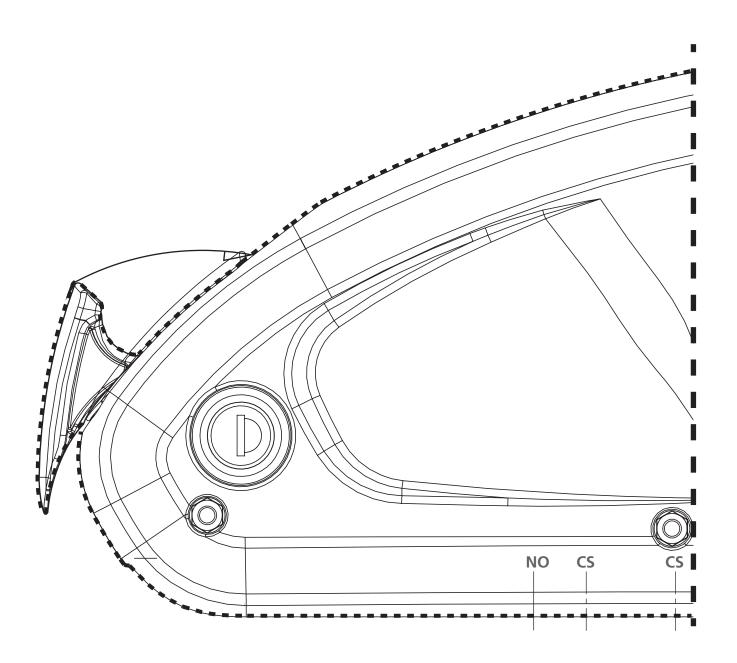
Cut out the battery template, use the markings over the bottle cage holes on the bicycle frame. The flat holes must be used together, the countersunk holes with the corresponding countersunk hole. Always attempt to use flat holes first. Leave 2.5cm (1") on the rear side (by the handle) for clearance when removing the battery.
