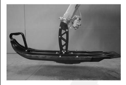
⇒ With the all bolts/fasteners fully tightened and the fork brace resting on the bottom of the fork the ski assembly should look similar to the image shown.
