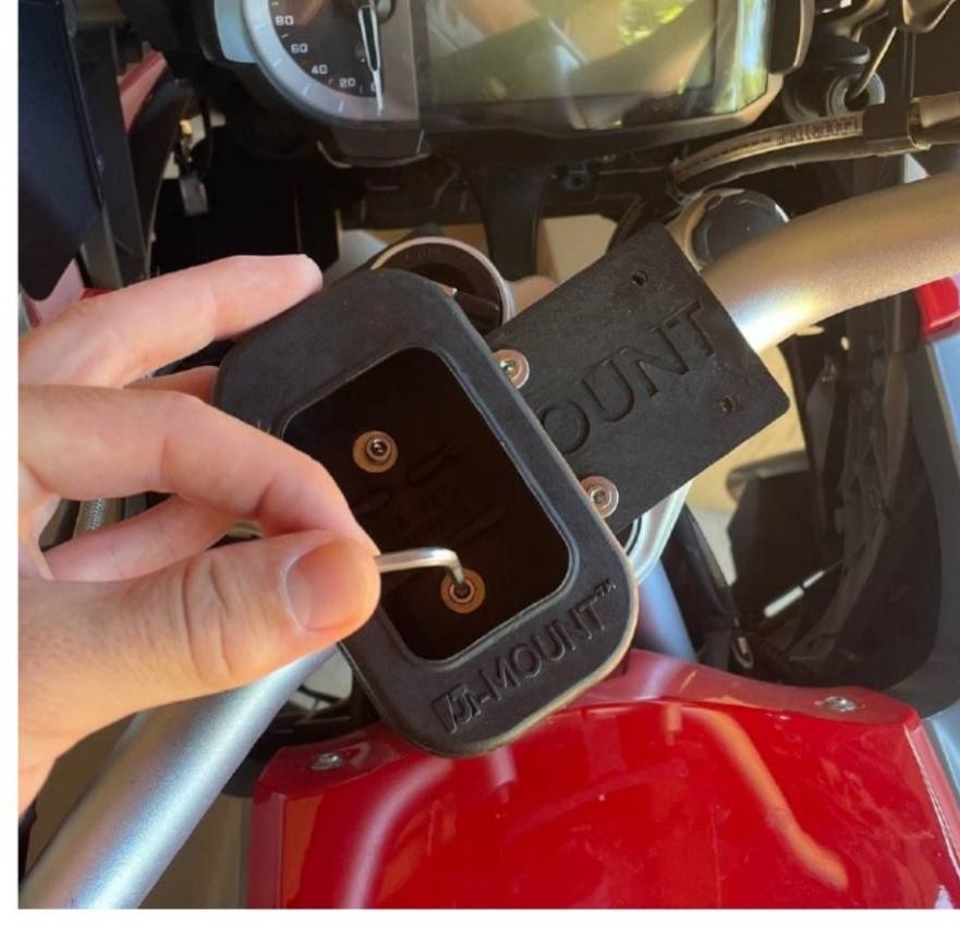
place the single mount in line with the cavities on either side of the baseplate and screw it down using the shorter screws
