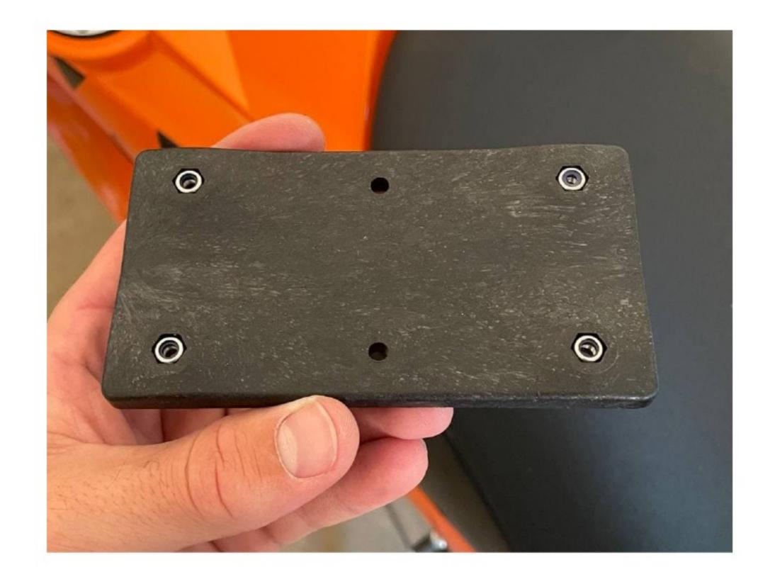
Press four nylock nuts into the cavities on the four corners of your base plate
