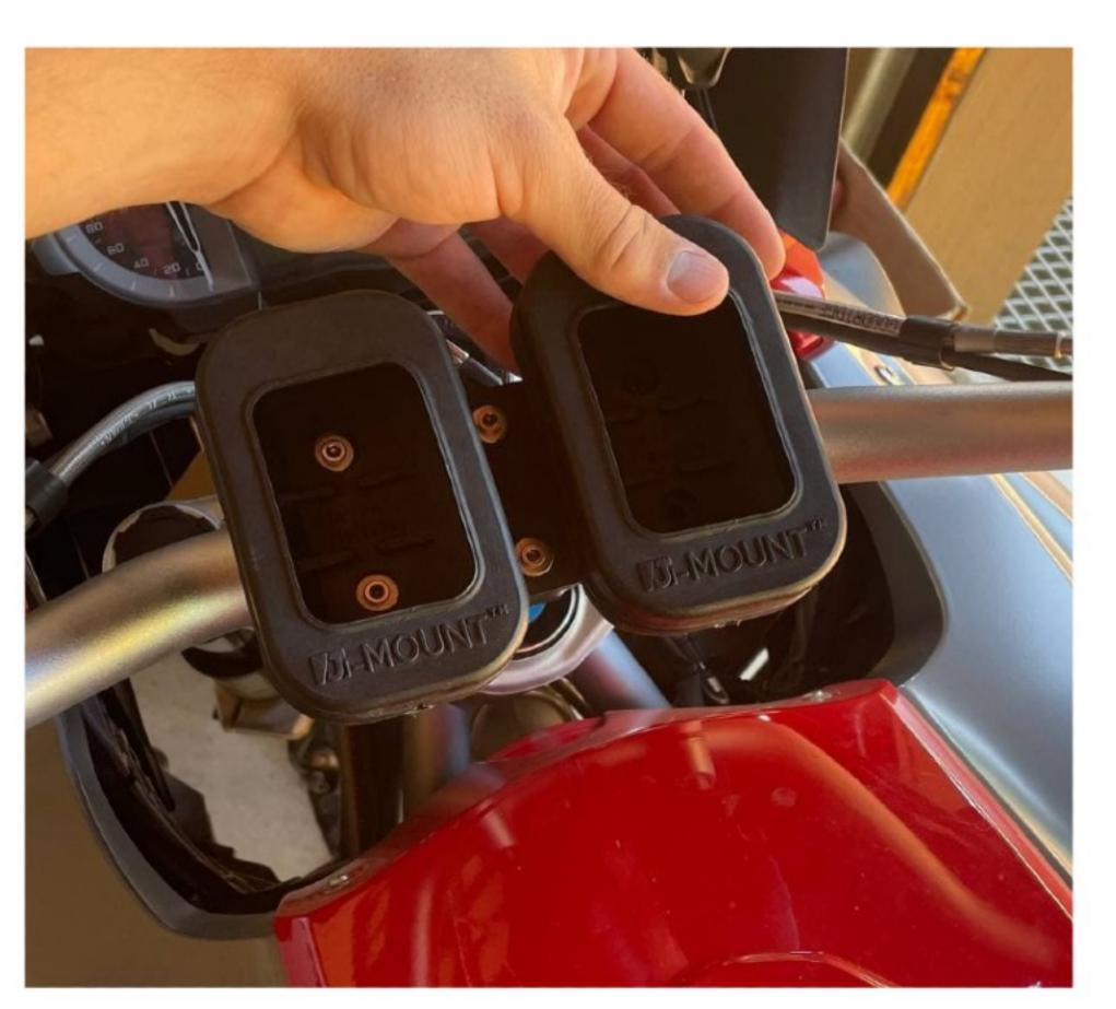
repeat on the other side with your second single mount NOTE: do not overtighten any of the screws a this will strip the cavities
