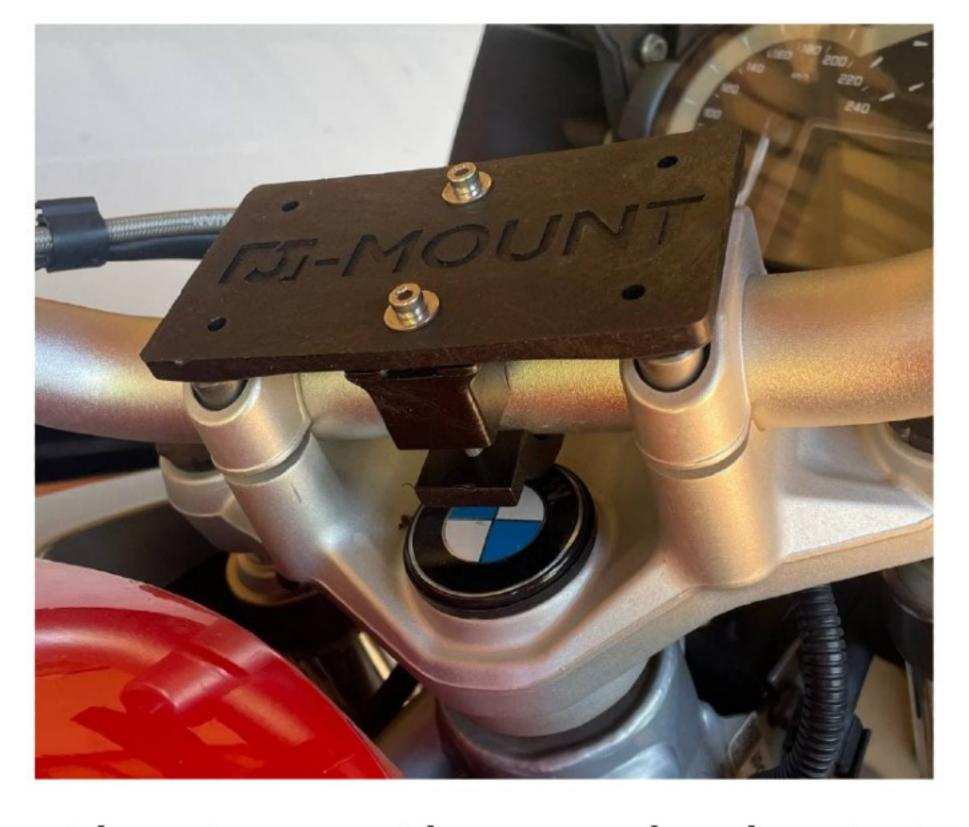
press the two other nylocks into the bottom piece of the handlebar clamp and evenly tighten the screws over the bars from the top
