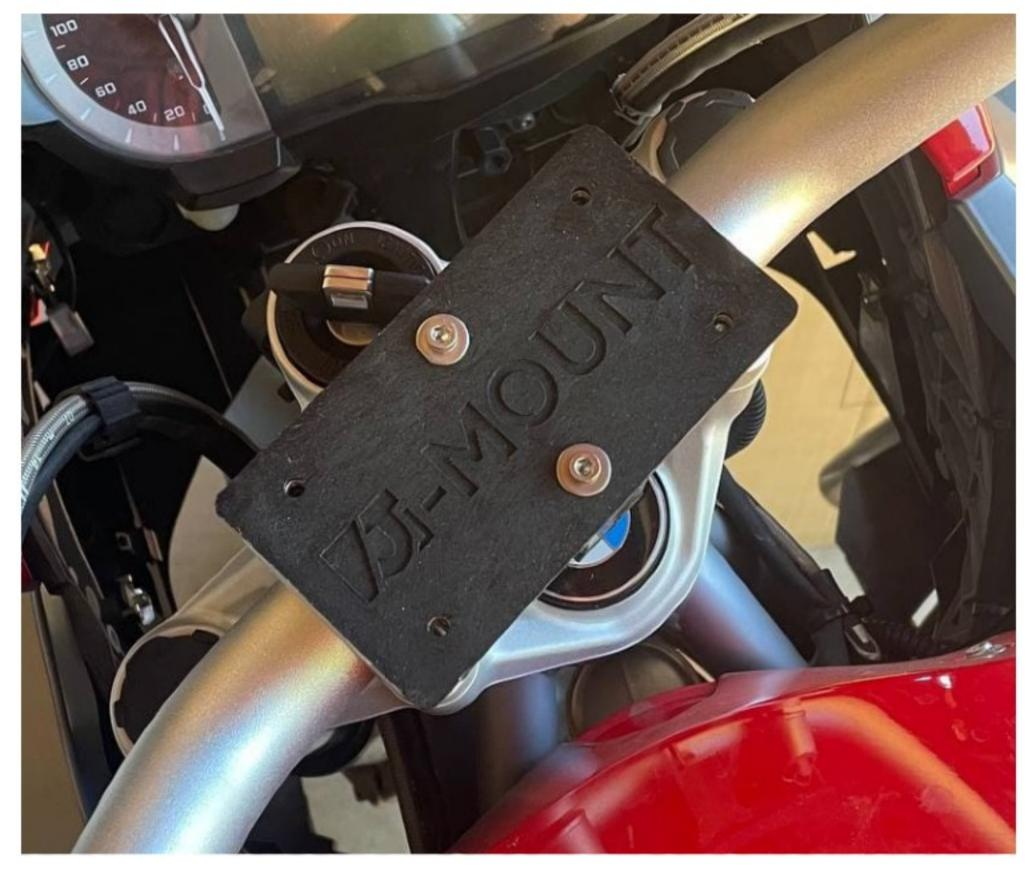
locate your baseplate in the desired location and then tighten it down evenly on both screws making sure not to overtighten
